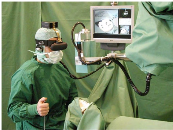
Figure 6: MINOP Telemanipulator platform for an electronic surgical microscope
