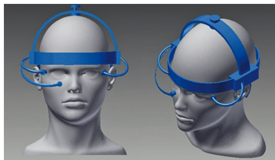
Fig. 13: Principle of the EEG-based Neurofeedback and conceptual design of the headset.
