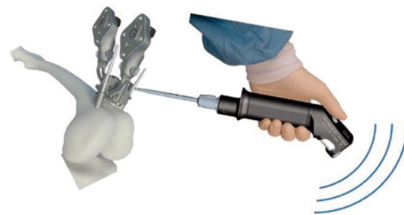
Fig. 10: Interactive computer controlled adjustment of a cutting guide for Total Knee Arthroplasty.
