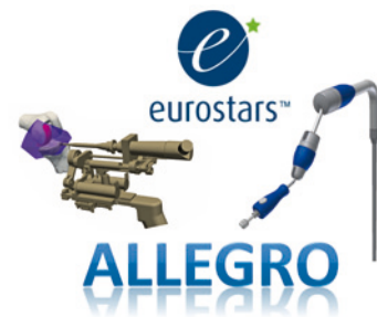
Fig. 9: Manipulator with milling tool for active path control in UKA and optional holding arm.
