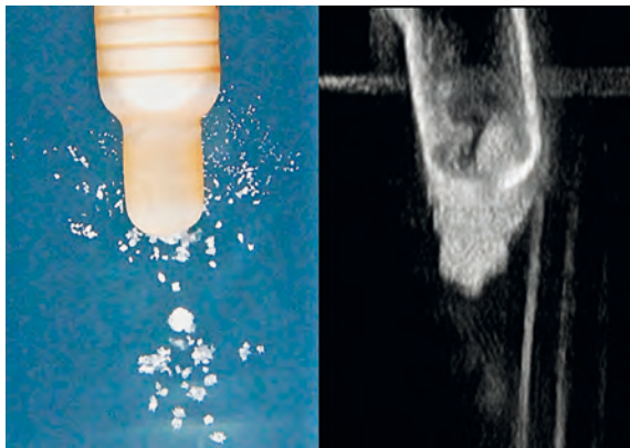
Fig. 8: Primary cavitation (left) and B-mode image of secondary cavitation (right).
