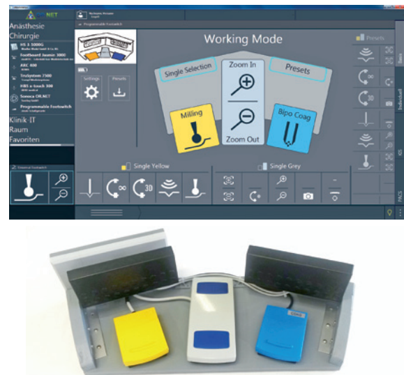
Fig. 12: Graphical user interface (upper) and first labtype of the integrated universal footswitch.
