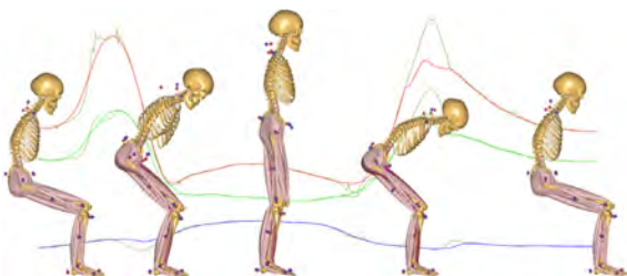
Fig. 1: Hip joint force evaluation for the process of getting up from a chair and sitting down again
