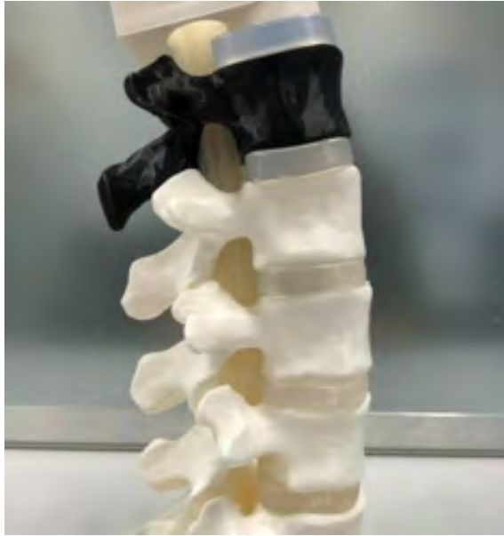
Fig. 3: In vitro model of the lumbar section of the spinal canal with intervertebral discs and nerve fibers.
