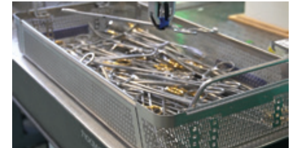
Fig. 5: Robotic picking of contaminated surgical instruments.
