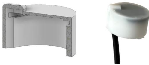
Fig. 7: CAD design and 3D printed transducer
