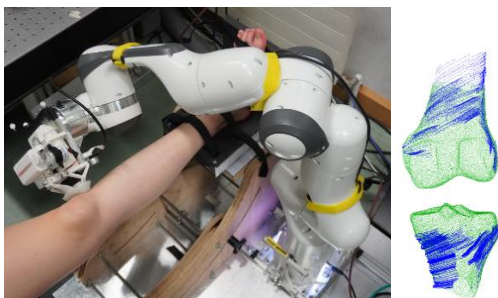
Fig. 4: Robotic Ultrasound System - 3D Knee Reconstruction.
