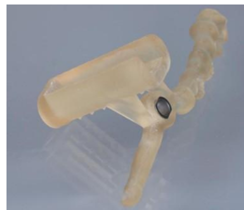
Fig. 6: PSI with integrated US probe holder
