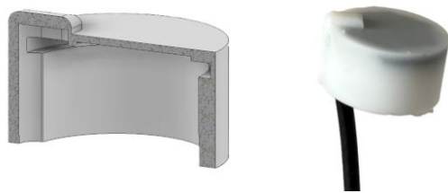
Fig. 7: CAD design and 3D printed transducer
